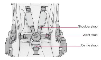
Feed the centre strap with the buckle between the child's legs. Then insert the buckle adaptors on the shoulder and waist straps from above into the top of the buckle. They should click audibly into position.
