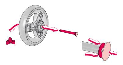
Guide the axle through the hub from the front of the wheel. Press on the cover until it snaps into position.
