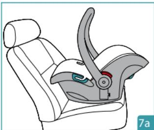
Place the child restraint rear-facing on the vehicle seat and make sure the handles in specified position. The child will face the rear of the vehicle.
