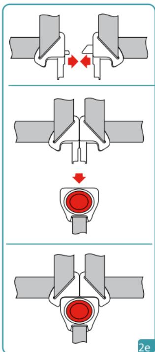
Put the two buckle tongues together, then lock into the female buckle. (2e)
