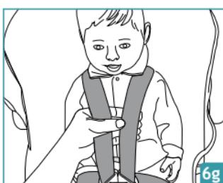
For proper tightness, one finger should fit between the harness straps and the child's shoulders.
