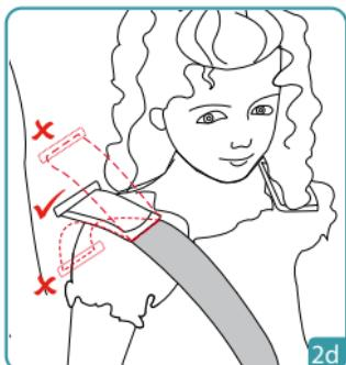
Position the height of harness according to the child's height. The harness straps should be level with the child's shoulders. Do not use the child restraint with the harness if the child's shoulder are above the heightest slots in the backrest or if the child's weight exceeds 13kg.
