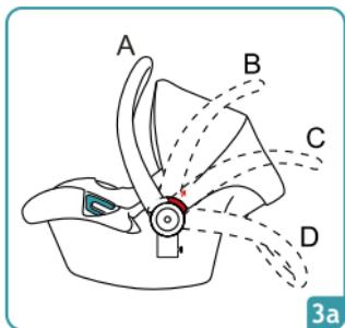
There are 4 positions: In vehicle position (A), Carry position (A), Middle position (B,C), and Stationary position(D).
