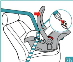
Route the vehicle lap belt through both lap belt guides and buckle the seat belt.
