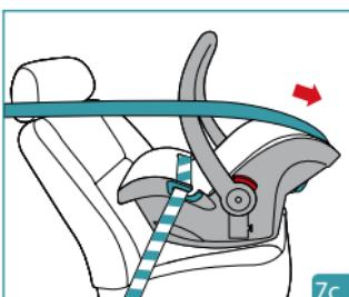
Route the vehicle shoulder belt around the back of the child restraint and through the shoulder belt guide.
