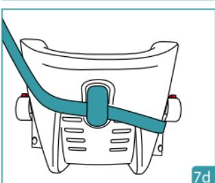
If vehicle shoulder belt is too short, please move vehicle seat belt height adjustment to the lowest possible height. If the vehicle belt is still too short, try another seating position.
